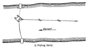
FIGURE 23.—Current operated ferries.
